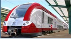
Electric Multiple Unit
